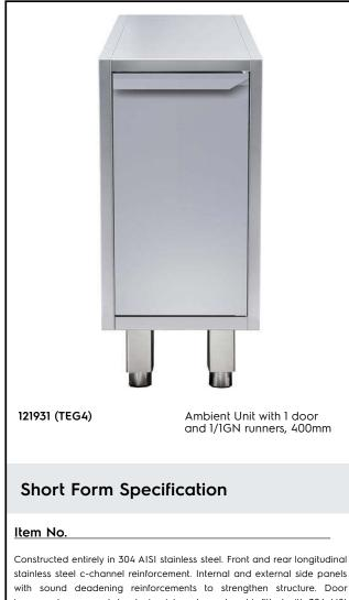
such as the control of the strengthener structure. Door incorporates a sound deadening reinforcements to strengthen structure. Door incorporates a sound deadening internal panel and is fitted with 304 AISI stainless steel hinges allowing an opening of 180° degrees. 150mm heightadjustable (0/+90mm) oversized feet (65x65mm) can be removed for masonry installation. 45° degree internal side corner junction system. 304 AISI stainless steel quide runners GN 1/1.
